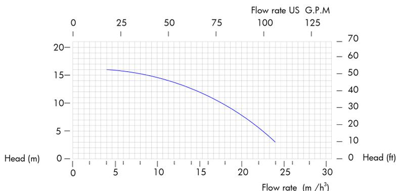
The curves and performance values refer to pumps with free delivery outlet with water at 20 °C, and two poles motor 50 Hz. These data may vary according to the construction materials and hydraulic conditions.
