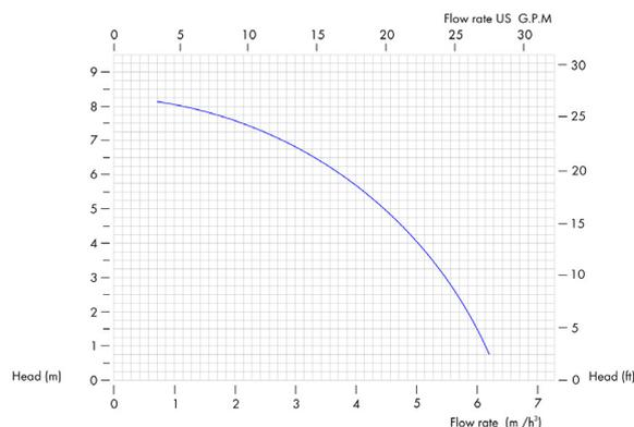
The curves and performance values refer to pumps with free delivery outlet with water at 20 °C, and two poles motor 50 Hz. These data may vary according to the construction materials and hydraulic conditions.
